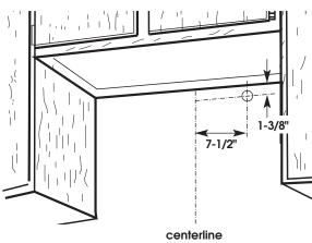
To wire through rear, mark a line 7-1/2" from the right of the centerline on the wall. Mark the point on this line that is 1-3/8" from underside of cabinet.
